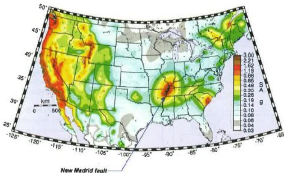
Figure 2 USGS seismic risk map. Colors indicate predicted seismic loads in terms of G force. Source: U.S. Geological Survey
